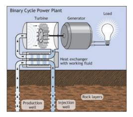
The efficiency of a binary plant is comparably low and economics questionable at low temperatures. That is why binary plants are often constructed together with a district heating system as cogeneration plant. In Europe binary plants often are rather small plants, often in sizes less than one megawatt.
